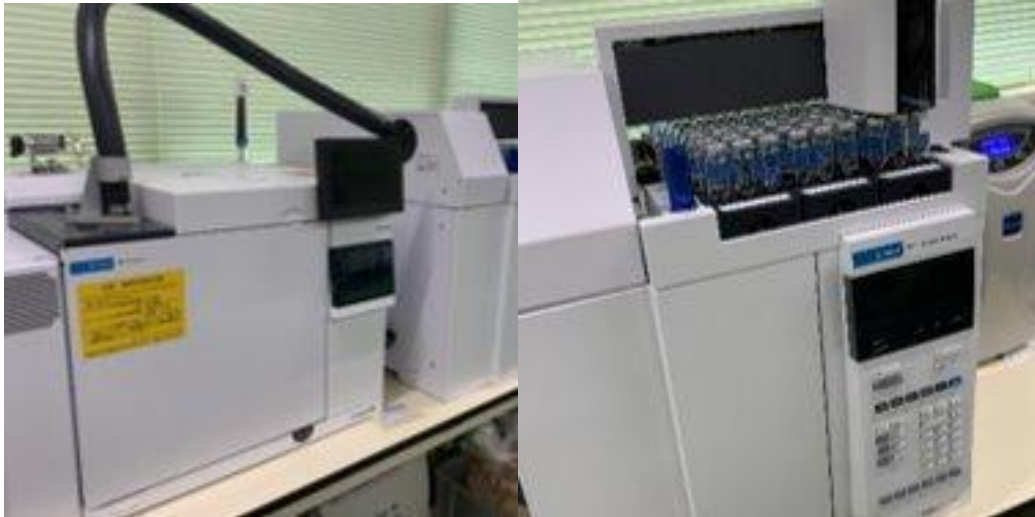
Figure 25 [Equipment for Methane Measurement Installed at the Faculty of Food and Agricultural Sciences, Fukushima University]
